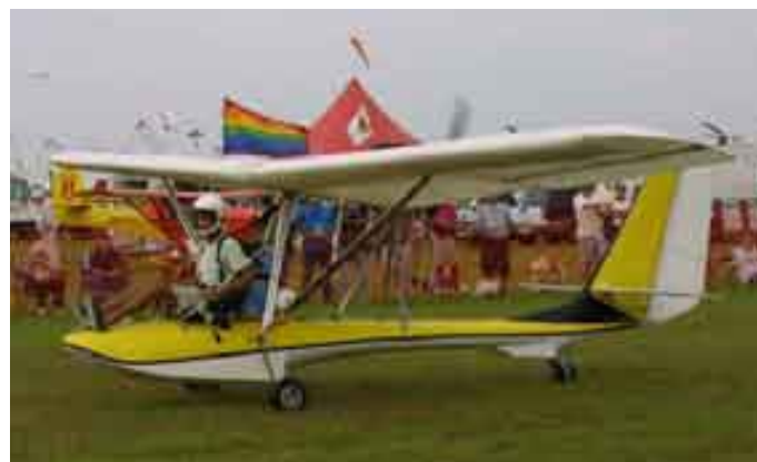
The Moyes Microlites Connie amphibious ultralight aircraft is an amphibious single centre float ultralight, with wing tip floats on the wings. . The pilot sits in front of the wing, in a seat on top of the float. The single lever retract system retracts the two main wheels and the tail wheel in one quick and easy motion.
