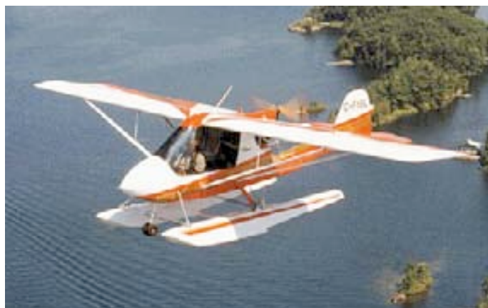
A quad City Challenger on Floats - similar to the one Steve Ridley operates
