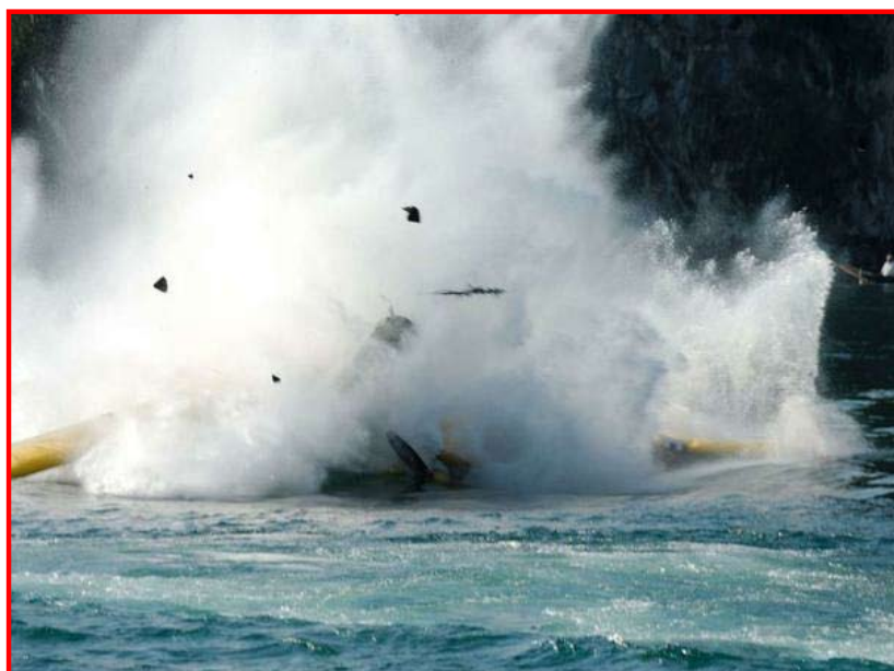
This "accident" resulted from a very flat high speed approach. The aircraft touched the water much too fast. The two black airborne objects are the float tip bumpers!
